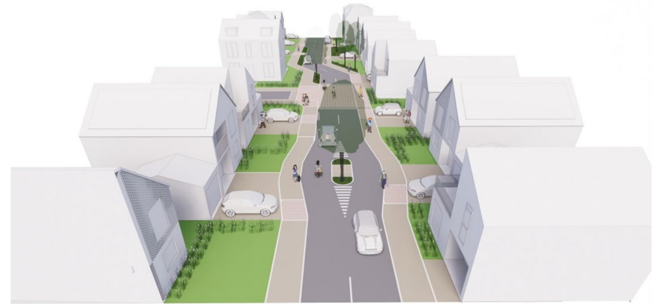
Figure 29 – Street Typology Section for a Local Street in a Coastal Context
