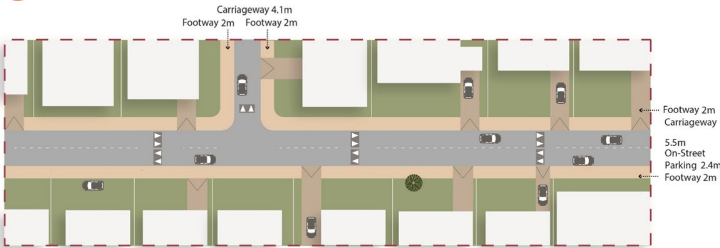
Figure 33 – Street Typology Plan for a Poorly Designed Residential Link Street in a Rural Context
