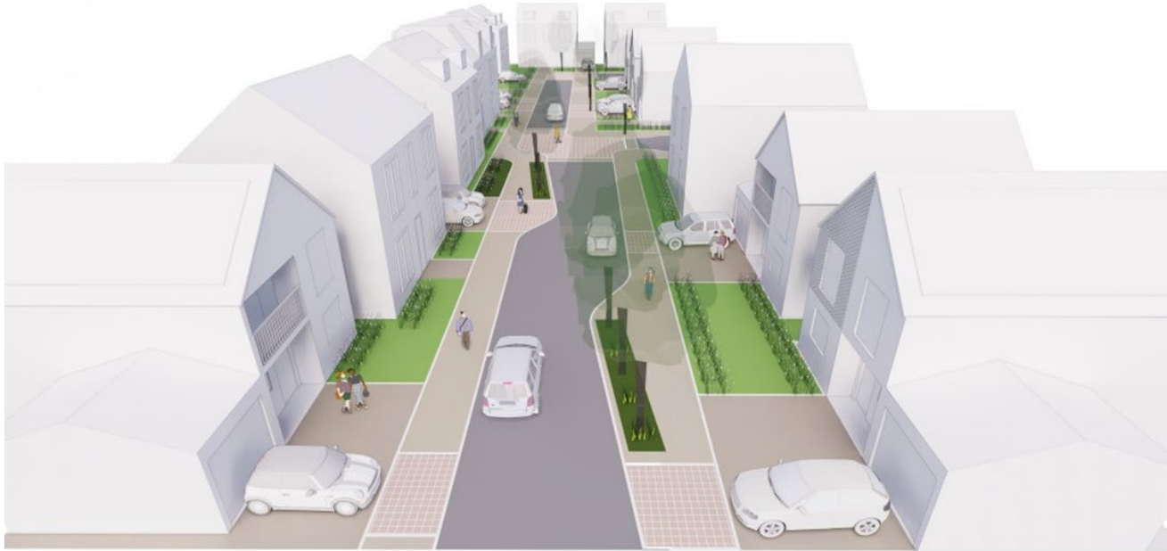
Figure 32 – Street Typology Section for Residential Link Street in a Rural Context
