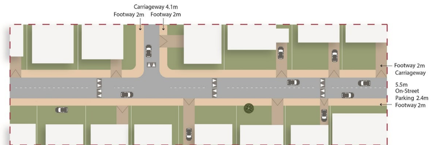
Figure 30 – Street Typology Section for a Poorly Designed Local Street in a Coastal Context
